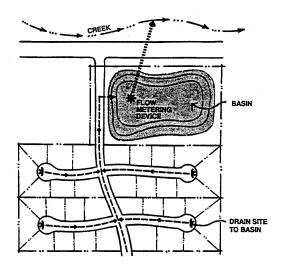
THE PRIMARY FUNCTION OF A DETENTION BASIN IS TO CONTROL THE RATE AT WHICH STORM WATER IS RELEASED FROM A DEVELOPMENT SITE. IN TEMPLETON, DETENTION IN THE UPPER REACHES OF TOAD CREEK WILL HELP TO PREVENT FLOODING IN THE LOWER REACHES. BASINS CAN PROVIDE DUAL USE FACILITIES: CAN BE USED FOR PARKS, BALLFIELDS OR OPEN SPACE. Guideline III.E.7: Site Grading
