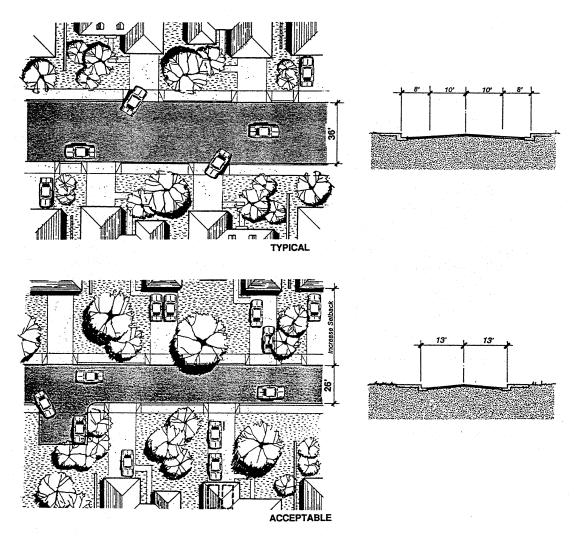
Reduce curb-to-curb street width from 36 to 24 feet for typical 50 ACT to 1500 ADT road section. Best suited to short loop roads where little through traffic can be expected.
